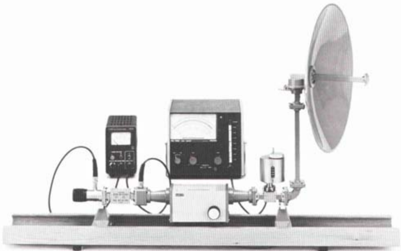
Experiment set-up with parabolic antenna.
